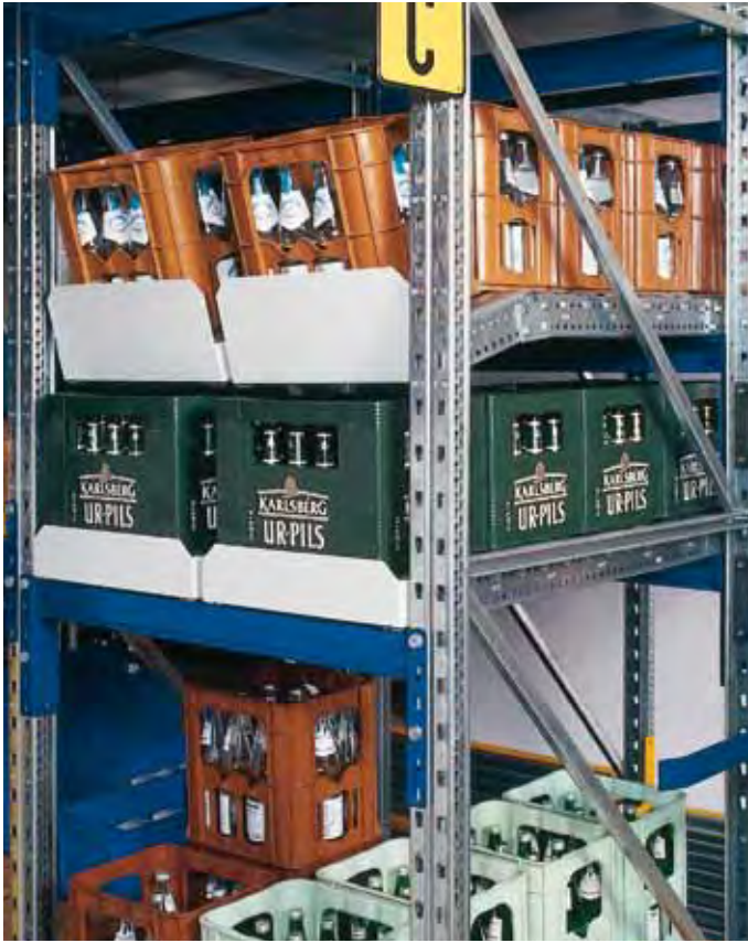
Lanes with inclined picking tray facilitate picking of individual bottles, straight lanes are suited for picking complete cases.
