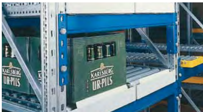
The loading side of the lanes is equipped with a push-back stop which tilts into the lane for ease of replenishment.
