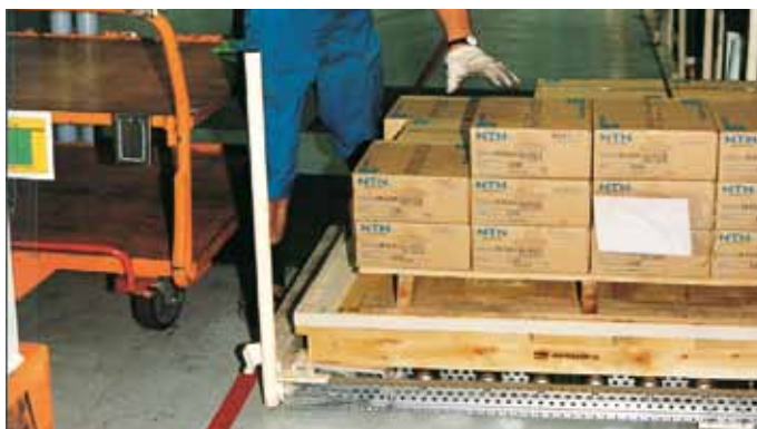
Extractable first pallet position, BITO-type »APP«
